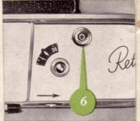
complete the transport movement. This at the same time tensions the shutter, and advances the film and the film counter (see also page 13).
