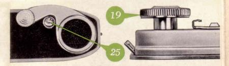
To rewind the exposed film, depress the reversing button (25) in the base of the camera and half pull out the rewind knob (19) (to its first stop) to get at it more easily. Then turn the rewind knob in the direction of the arrow until the reversing button ceases to rotate. This is easily observed by the small black dot near the rim of the button.
